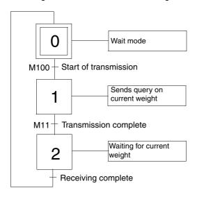
The terminal functions as a master system for the weighing system, i.e. it continuously asks for the current weight. The connections between the controller, terminal and weighing system are shown in the figure below.
