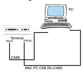
To connect the controller to the terminal, use the cable recommended in the driver manual for the selected controller.
