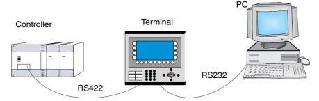
Terminal connected to the programming/printer port.
