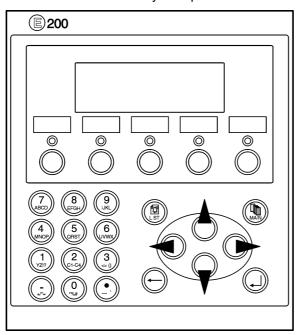
The terminals have a different number of built-in function keys, depending on the terminal model.
