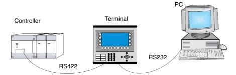
Terminal connected to the programming/printer port.
